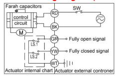
**VALVE OPEN**: Black wire connects to Negative and Red wire connect to Positive, valve Open.
