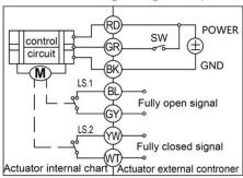
**VALVE OPEN**: Black wire connect to Negative and Red wire connect to Positive, meanwhile Green wire connects to Positive, valve Open.
