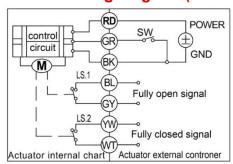
**VALVE OPEN**: Black wire connects to Negative and Red wire connects to Positive, meanwhile Green wire connects to Negative, valve open.
