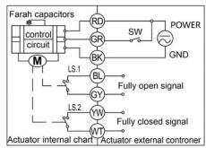
**VALVE OPEN**: Black wire connect to Negative and Red wire connect to Positive, meanwhile Green wire connects to Positive, valve Open.
