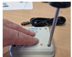
4. Open the controller carefully, do not pull apart as there are two small wires connecting the base and circuit board. (see yellow arrow)
