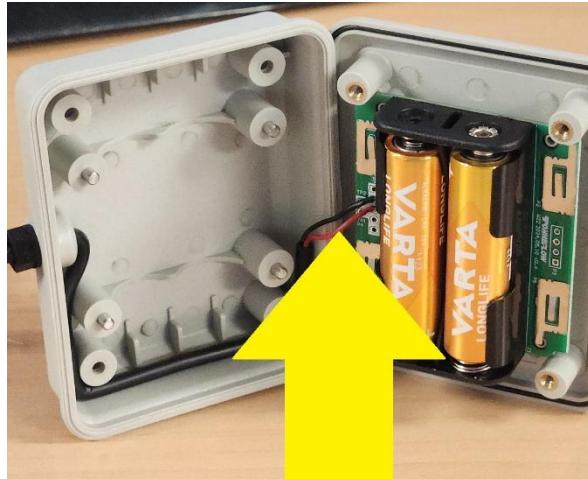
5. Replace the two AA batteries with good quality long lasting lithium batteries. (Battery -ve against spring). We recommend VARTA LONGLIFE LOW USE AA, Reference: 4106301124
