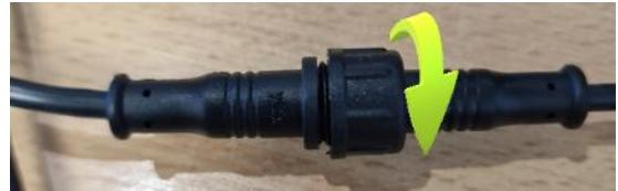
2. Note that the plug ends will only fit back together one way.
