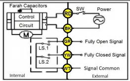
Power ON motor actuates valve into powered position and then automatically powers off. Valve stays in powered position.
